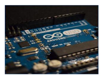
The Atmega-328P-based Arduino Uno is a development board for microcontrollers.
